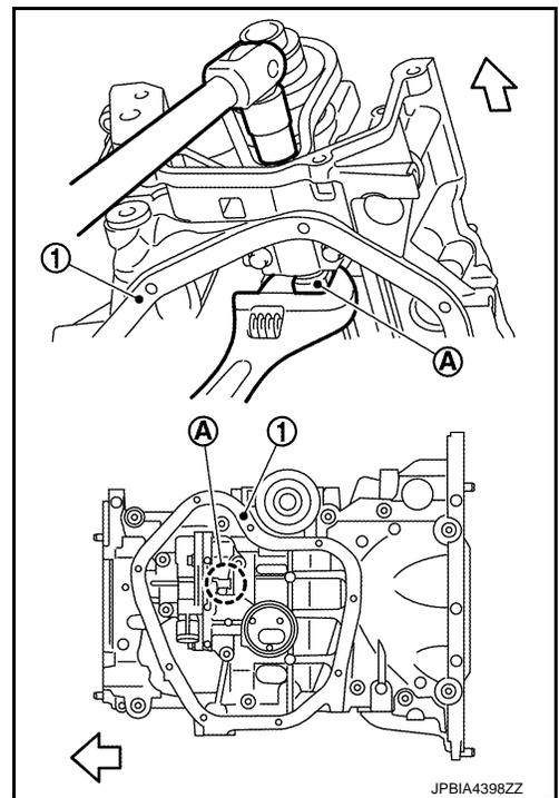
5. Install oil pump chain tensioner (1).
