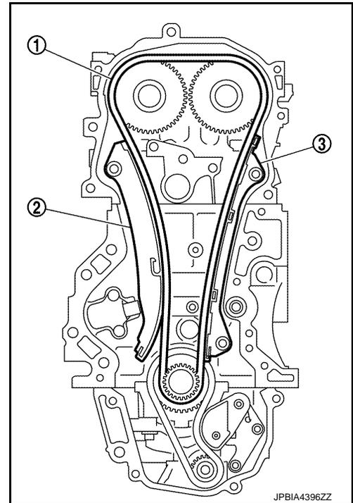
13. Remove crankshaft sprocket and oil pump drive component with the following procedure:
