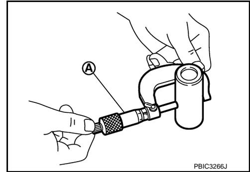
Piston to Piston Pin Oil Clearance
