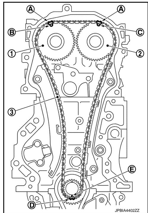
7. Install the slack guide (2) and the tension guide (3).
