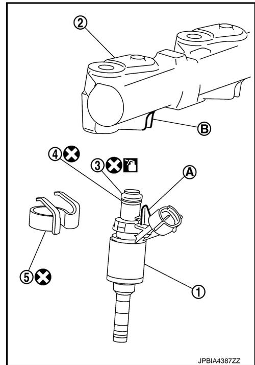
4. Install fuel rail and fuel injector assembly to cylinder head.
