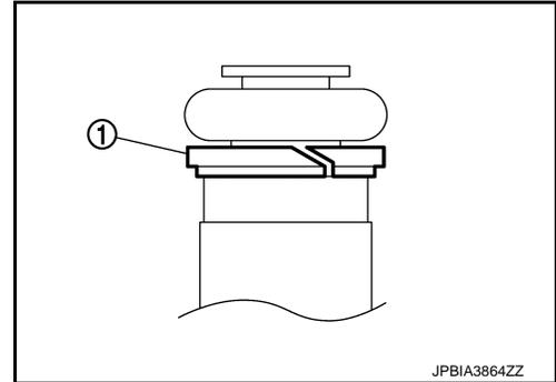
3. Install fuel injector (1) to fuel rail (2) as per the following:
