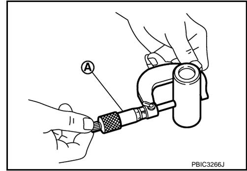
Connecting Rod Bushing Oil Clearance
