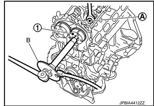
5. Install timing chain and related parts. Refer to [EM-72, "Exploded View"](#).
