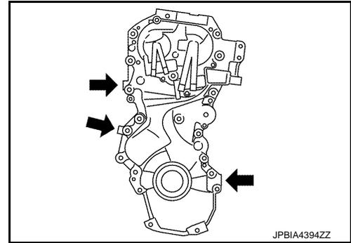
9. Remove front oil seal from front cover.
