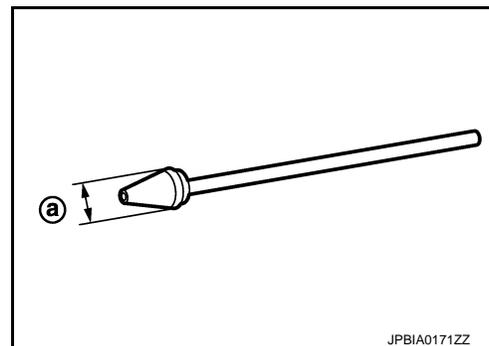
6. With accelerator pedal fully depressed, turn ignition switch to "START" for cranking. When the gauge pointer stabilizes, read the compression pressure and the engine rpm. Perform these steps to check each cylinder.
