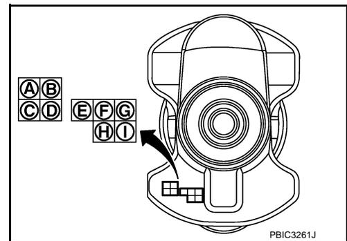
3. Read the symbol at the cross point of selected row and column in the "Connecting Rod Bearing Selection Table".
