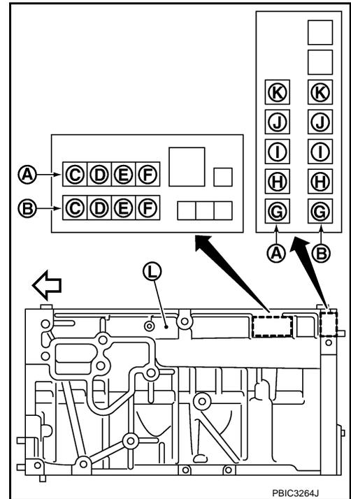
2. Apply main journal diameter grade stamped on crankshaft front side to column in the "Main Bearing Selection Table".
