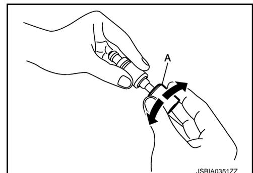
2. Install O-ring and backup ring to fuel injector. When handing new O-ring and backup ring, paying attention to the following caution items:
