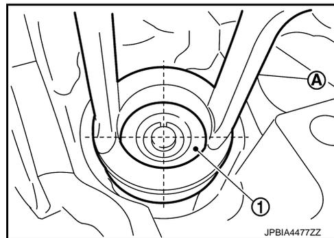
4. Remove valve spring retainer and valve spring (with valve spring seat).
