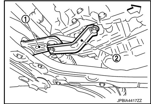
5. Remove stabilizer connecting rod. Refer to [FSU-14, "Exploded View"](#).
