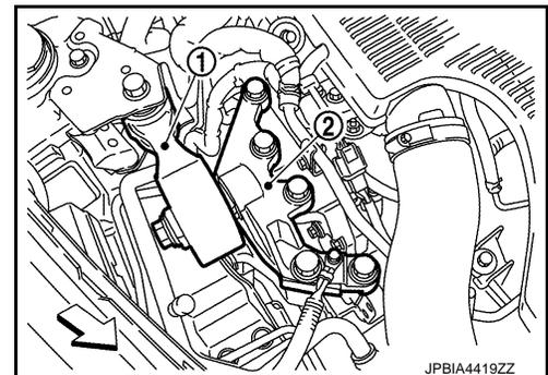
3. Remove engine mounting insulator (LH).
