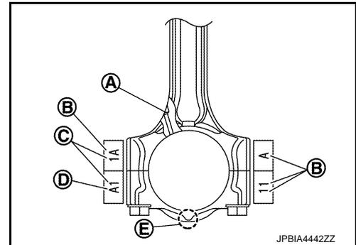
2. Apply crankshaft pin journal diameter grade stamped on crankshaft front side to the column in the "Connecting Rod Bearing Selection Table".
