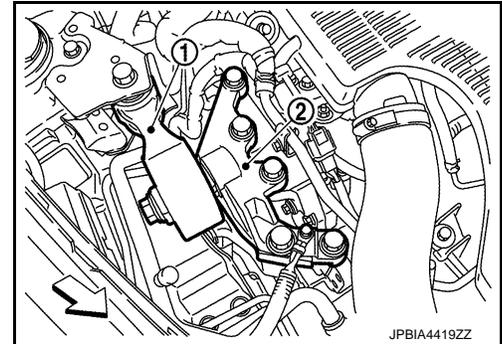
3. Remove engine mounting insulator (LH). (CVT models)
