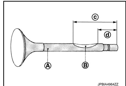
3. Use hacksaw to cut through approximately half the diameter of valve stem. Make the serration at a point 40 mm (1.57 in) from the end of valve stem.
