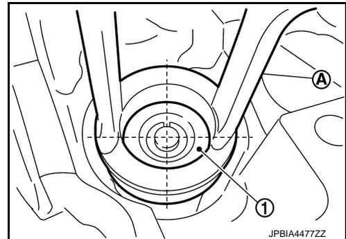
5. Remove valve spring retainer and valve spring (with valve spring seat).
