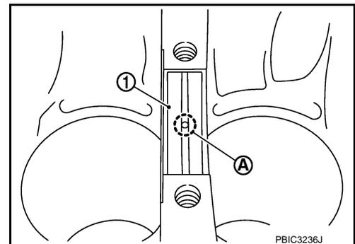
4. Install signal plate to crankshaft if removed.
