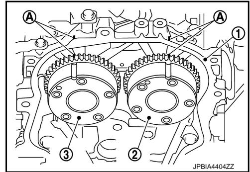
4. Remove camshaft sprockets (INT and EXH).
