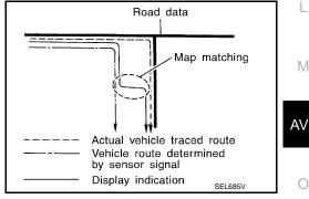
The vehicle position may not be corrected under the following circumstances and after driving for a certain time when GPS information is difficult to receive. In this case, the vehicle mark on the display must be corrected manually.
