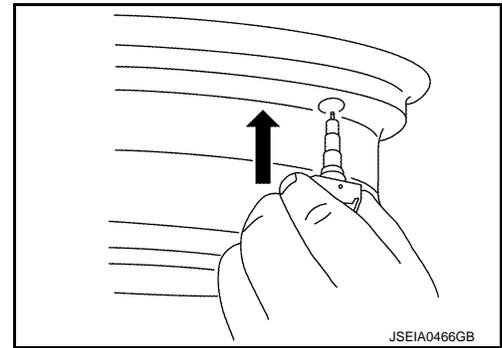
5. Set the tire onto the turntable so that the tire changer arm (2) is at a position approximately 270° from the tire pressure sensor (1).
