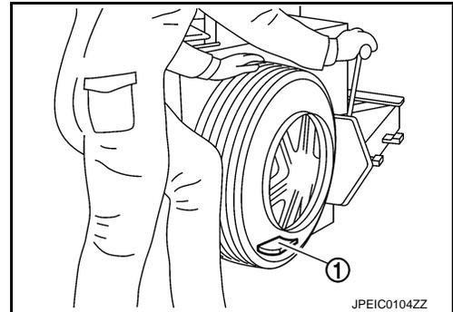
7. Turn tire so that valve hole is at bottom and bounce so that tire pressure sensor (1) is near valve hole. Carefully lift tire onto turntable and position valve hole (and tire pressure sensor) 270 degree from mounting/dismounting head (2).
