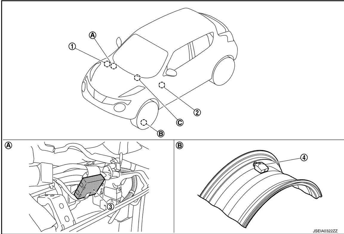
1. ABS actuator and electric unit (control unit)
