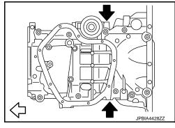
Insert seal cutter [SST: KV10111100 (J-37228)] between oil pan (upper) and cylinder block, and slide it by tapping on the side of the tool with a hammer.
