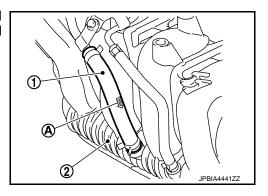
**Electric Throttle Control Actuator**
