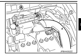
Remove the air cleaner filter (1) and air cleaner body (2) from the air cleaner case.
