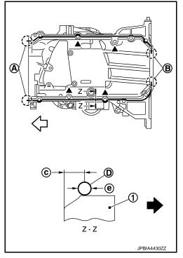
c. Install new O-ring at cylinder block side.
