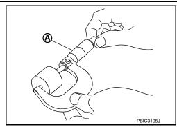
Measure the thickness of the replacement valve lifter using the following formula. (Units: mm)
