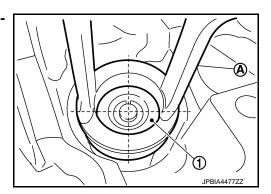
Remove valve spring retainer and valve spring. CAUTION:
