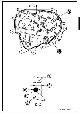
Tighten bolts in the numerical order shown in the figure. NOTE:
