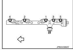
14. Remove fuel injector from cylinder head as per the following.
