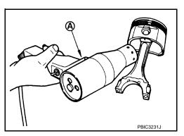
c. Push out piston pin with stick of outer diameter approximately 18 mm (0.71 in).
