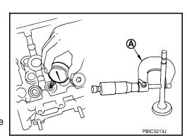
• If the calculated value exceeds the limit, replace valve and/or valve guide. When valve guide must be replaced. Refer to EM-101, "Disassembly and Assembly".
