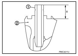
d. Apply reamer finish to valve guide with a valve guide reamer (commercial service tool) (A).
