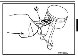
b. Heat piston to 60 - 70°C using an industrial dryer (A).
