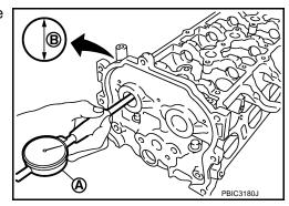
How to calculate camshaft oil clearance
