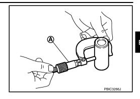
Connecting Rod Bushing Oil Clearance
