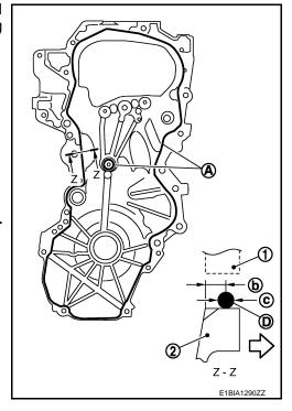
b. Install the O-ring into the cylinder block mounting groove.
