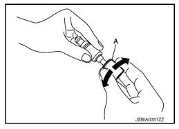
2. Install O-ring and backup ring to fuel injector. When handing new O-ring and backup ring, paying attention to the following caution items:
