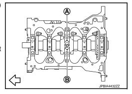
b. Tighten main bearing cap bolts in numerical order as shown in the figure with the following procedure:
