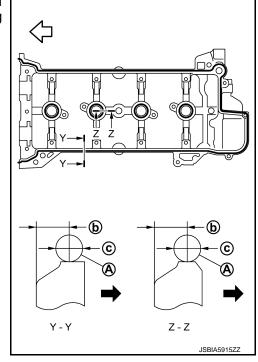
c. Tighten camshaft bracket bolts evenly in three steps in the order as shown in the figure.
