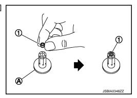
Straightly insert seal ring (1), which is set in step 2, to fuel injector as shown in the figure and install.
