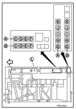
Apply main journal diameter grade stamped on crankshaft front side to column in the "Main Bearing Selection Table".
