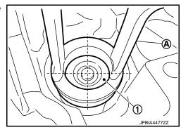
5. Remove valve spring retainer and valve spring (with valve spring seat). **CAUTION:**
