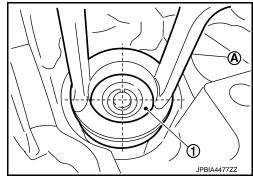
Remove valve spring retainer and valve spring (with valve spring seat).
