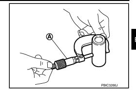
Piston to Piston Pin Oil Clearance
