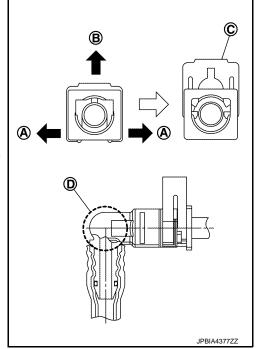
To prevent damage to each joint and protect it from the entry of foreign matter, cover the joint with plastic bag (A) or an equivalent.
