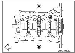
7. Tighten main bearing cap bolts in the numerical order shown in the figure with the following steps.
