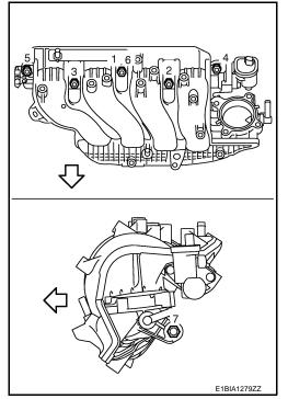
12. If necessary, remove the EVAP purge control solenoid valve from the intake manifold.
