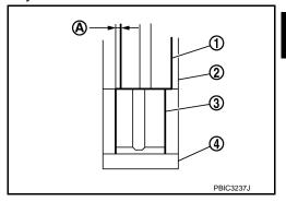
• Check that the oil hole in cylinder block and the oil hole (A) in main bearing (1) are aligned.
