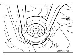
Remove valve spring retainer and valve spring. CAUTION:
