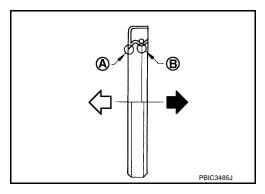
Press-fit the rear oil seal using a drift (commercial service tool) with outer diameter of approximately φ115 mm (4.5 in) and inner diameter of approximately φ90 mm (3.5 in), with the following precautions in mind.
