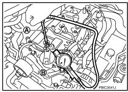
Use the adapter whose picking up end inserted to spark plug hole is smaller than 20 mm (0.79 in) in diameter. Otherwise, it may be caught by cylinder head during removal.
