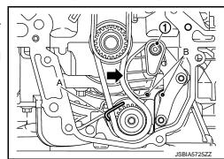
EM-251 Revision: 2014 October 2015 JUKE d. Hold the oil pump shaft end (A), and then loosen and remove the oil pump sprocket mounting nut (B).
