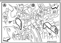
Remove starter motor. Refer to STR-26, "MR16DDT: Removal and Installation".
