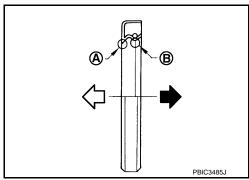
• Press-fit front oil seal using a suitable drift with outer diameter 57 mm (2.24 in) and inner diameter 45 mm (1.77 in).
