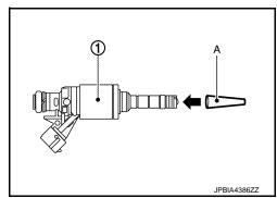
b. Set seal ring (1) to injector seal drift set [SST: KV101197S0 (—)] (A).
