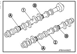
• Install camshafts to the cylinder head so that knock pin (A) on front end is positioned as shown in the figure.
