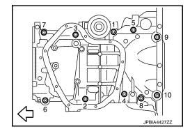
Insert a screwdriver shown by the arrow (←) in the figure and open up a crack between oil pan (upper) and cylinder block.
