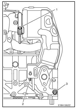
3. Follow the procedure below and install the catalyst converter adapter.
