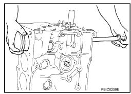
Remove connecting rod bearings.
