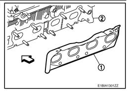
Tighten nuts in the numerical order shown in the figure.
