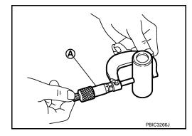
Calculating connecting rod small end clearance
