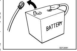
After installing the 12V battery, always check "Self Diagnosis Result" of all ECUs and erase DTC.
