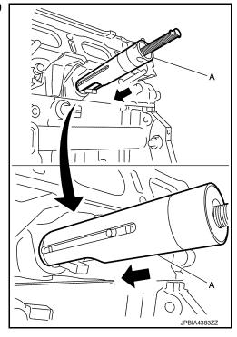
d. Tighten injector remover [SST: KV10119600 (—)] clockwise and remove injector from cylinder head.
