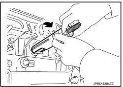
e. Pinch the seal ring (1) and cut it off. Never scratch the fuel injector.
