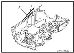
b. Apply a continuous bead of liquid gasket (D) with a tube presser (commercial service tool) as shown in the figure.
