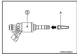
b. Set the seal ring (1) onto the injector seal drift [SST: KV101197S0 ( - )] (A).
