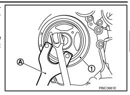
Attach a pulley puller [SST: KV11103000 ( — )] (A) in the M6 thread hole on crankshaft pulley (1), and remove crankshaft pulley.
