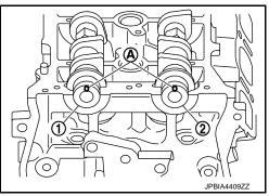
3. Install camshaft bracket with the following procedure:
