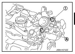
Connect fuel feed hose with the following procedure, and them install the fuel feed hose.
