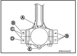
Apply crankshaft pin journal diameter grade stamped on crankshaft front side to the column in the "Connecting Rod Bearing Selection Table".
