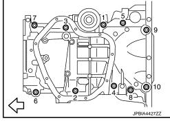
Insert a flat-bladed offset screwdriver or an equivalent into the location shown by the arrow (←) in the figure, and open up a clearance between the oil pan (upper) and cylinder block.
