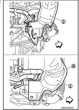
2. Start the engine and increase the engine speed. Check for exhaust gas and coolant leakage.
