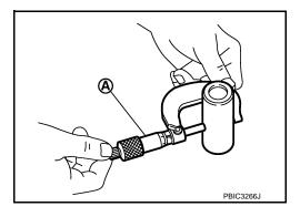
How to calculate piston-to-piston pin clearance
