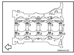
Turn main bearing cap bolts 70 degrees clockwise (angle tightening) in order from No. 1 to 10 in the figure.
