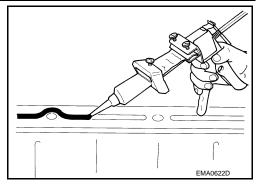
• As for bolt holes <sup>®</sup>, normally apply liquid gasket inside the holes. Occasionally, it should be applied outside the holes. Check to read the text of this manual.
