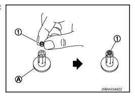
c. Install the seal ring (1) set in step 2 by inserting it straight into the fuel injector as shown in the figure.
