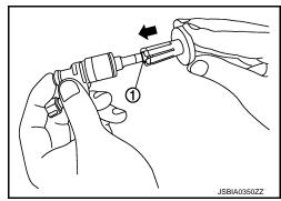
d. After installing the seal ring onto the fuel injector, install the injector seal drift [SST: KV101197S0 ( — )] (A) onto the fuel injector as shown in the figure. Turn it left and right by 90° at a time until it contacts the seal ring to settle the seal ring in place. **NOTE:**
