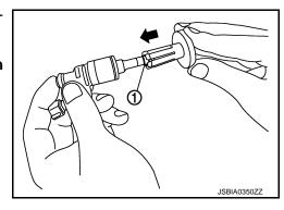
d. Insert injector seal drift set [SST: KV101197S0 (—)] (A) to injector and rotate clockwise and counterclockwise by 90° while pressing seal ring to fit it.
