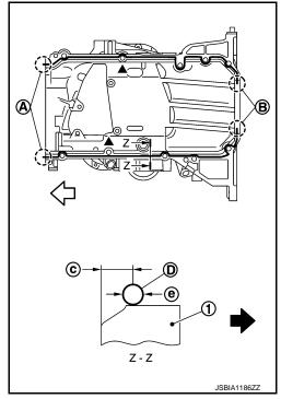
Install the O-ring into the installation groove on the cylinder block, and install the oil pan (upper) onto the cylinder block. Do not allow the O-ring to become displaced.
