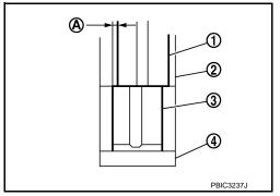
• Ensure the oil holes on cylinder block and oil holes (A) on the main bearings (1) are aligned.
