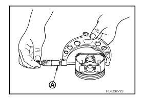
Piston to Cylinder Bore Clearance
