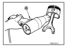
c. Using a round bar with outer diameter of approximately 18 mm (0.71 in), press out piston pin.
