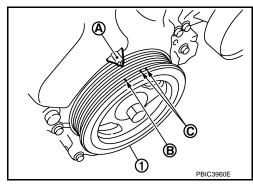
Check that the camshaft nose of cylinder No. 1 is positioned as shown in the figure.
