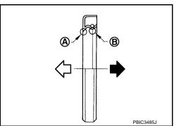
3. Press-fit the oil seal using a drift with outer diameter approximately \$67 mm (2.2 in) and inner diameter approximately  $\phi$ 45 mm (1.8 in) (commercial service tool). The oil seal front end surface should be within the following dimensions, with the front cover front end surface as the standard surface.
