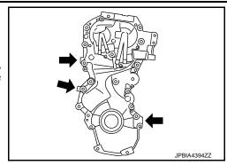
9. Remove front oil seal from front cover.
