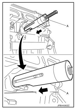
Tighten the injector remover [SST: KV10119600 ( — )] clockwise, and remove injector from cylinder head.
