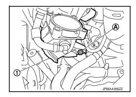
Loosen mounting bolts in reverse order as shown in the figure.
