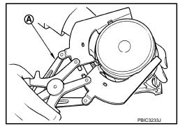
8. Remove piston from connecting rod according to the following procedure.
