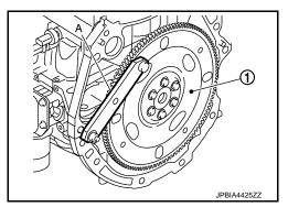
Remove pilot converter (1) (CVT models) or pilot bush (M/T models) using pilot bushing puller [SST: ST16610001 (J-23907)]
