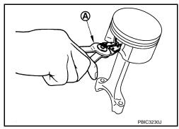
b. Heat piston to 60 to 70°C (140 to 158°F) with an industrial use drier (A) or equivalent.
