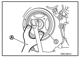
b. Loosen and pull out crankshaft pulley bolts.
