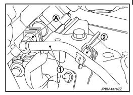
Disengage (A) and pull up (B) the pawl of the fuel feed hose connector retainer (C) to disconnect the fuel feed hose from high pressure fuel pump.
