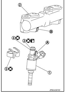
Install the fuel injector assembly into the cylinder head installation hole.
