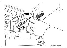
e. Cut seal ring (1) while pinching it. Be careful not to damage injector.
