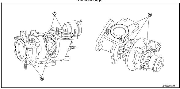
A. Check for leakage
