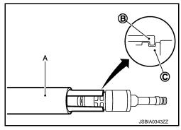
c. Press down body portion of injector remover [SST: KV10119600 (—)] (A) until it contacts cylinder head.
