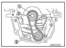
14. Remove the timing chain tension guide (front cover side) from the front cover if necessary.
