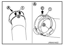
b. Move the spring upward and pull out the hose.
