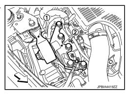
3. Remove engine mounting insulator (LH). (CVT models)
