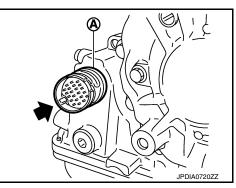
Press the CVT unit connector (A) into the transaxle case.
