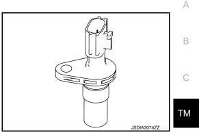
Ε The input speed sensor generates an ON-OFF pulse signal according to the rotating body speed. TCM judges the rotating body speed from the pulse signal.
