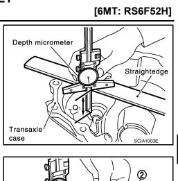
2. Using a depth micrometer and straightedge as shown, measure dimension (Q2) between clutch housing (1) end face and end face of reverse idler gear (rear) (2). **CAUTION:**
