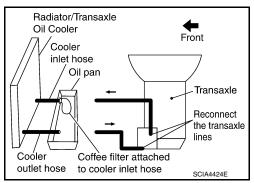
Radiator/Transaxle Oil Cooler Front Cooler inlet hose Coffee filter Transaxle Reconnect the transaxle lines Cooler Blow compressed outlet hose Oil pan air into outlet hose SCIA4425E
