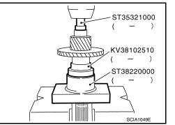
2. Press in 1st main gear bushing using Tools.
