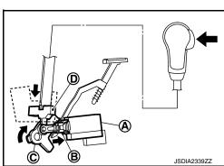
P POSITION HOLD MECHANISM (IGNITION SWITCH LOCK)
