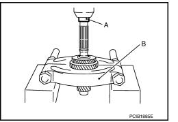
Remove snap ring. Remove C-ring holder and then remove mainshaft C-rings.
