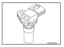
• The output speed sensor generates an ON-OFF pulse signal according to the rotating body speed. TCM judges the rotating body speed from the pulse signal.
