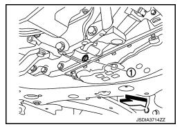
Install the charging pipe set (KV311039S0) (A) into the overflow plug hole.
