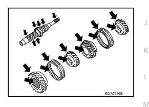
Synchronizer Hub and Coupling Sleeve
