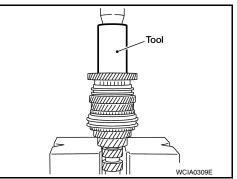
15. Install snap ring onto input shaft and make sure that end play (gap between snap ring and groove) of 6th input gear bushing satisfies the standard value.
