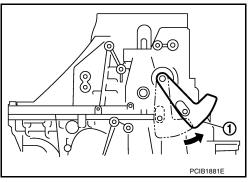
· When transaxle is shifted to the 1st gear position, mainshaft assembly (1) is declined.
