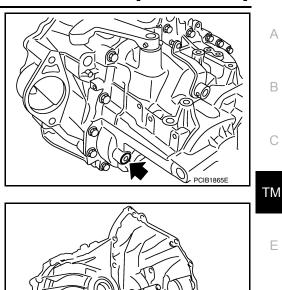
35. Install gasket onto drain plug and then install them into clutch housing. Tighten drain plug to the specified torque. CAUTION: Do not reuse gasket.
