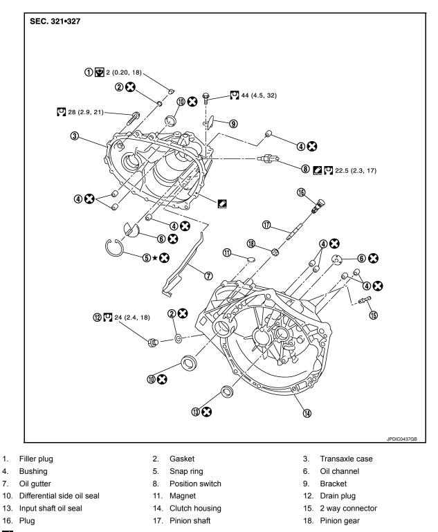
Apply Genuine Silicone RTV or an equivalent. Refer to <u>GI-22, "Recommended Chemical Products and Sealants"</u>.
