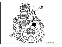
12. Install 3rd-4th shift fork (1) to 3rd-4th coupling sleeve.
