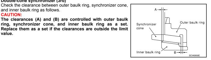
1. Measure the clearance (A) at 2 points or more diagonally opposite using a dial indicator. And then calculate mean value.
