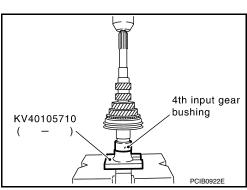
8. Select thrust washer so that dimension "C2" satisfies the standard value below. Then install thrust washer onto input shaft. Refer to <u>TM-145</u>, "Available Thrust Washer".
