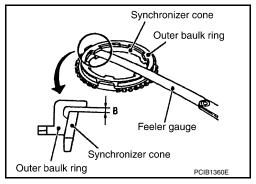
Measure the clearance (C) at 2 points or more diagonally oppo-3. site using a feeler gauge when pressing baulk ring toward clutch gear taper cone. And then calculate mean value.
