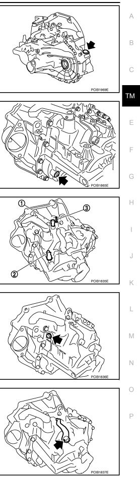
3. Remove plug and gasket from transaxle case.
