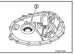
17. Remove differential side bearing outer race (1) from clutch housing, using a brass rod.
