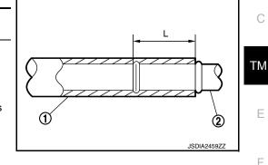
Refer to the followings when installing hose clamp. **CAUTION:** Hose clamp should not interfere with the bulge of tube.
