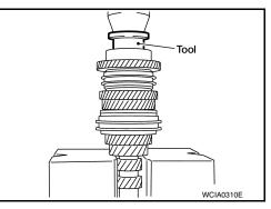
17. Press in input shaft front bearing using Tools.
