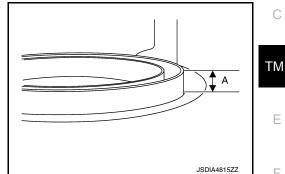
Parallelism at four diagonal points (➡) CAUTION: The difference among four diagonal points must be within 0.3 mm (0.012 in). NOTE:
