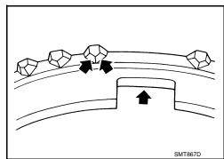
• If any crack, damage, or excessive wear is found on cam face of baulk ring or working face of insert, replace it.
