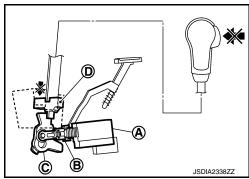
When brake pedal is depressed (selector lever operation allowed) The shift lock solenoid (A) is turned ON (energized) when the brake pedal is depressed with the ignition switch ON. The solenoid rod (B) is compressed with the electromagnetic force. The connecting lock lever (C) rotates when the solenoid rod is compressed. Therefore, the detent rod (D) can be moved. The selector lever can be shifted to other positions for this reason.
