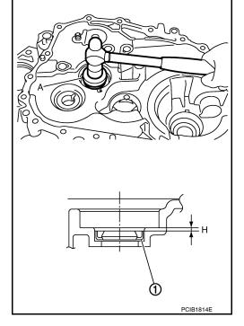
3. Install differential side bearing outer race (clutch housing side) to clutch housing using Tools.
