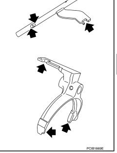
• Check if the width of shift fork hook (sliding area with coupling sleeve) is within allowable specification below.
