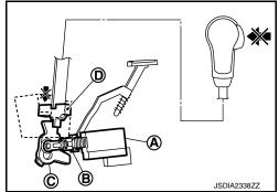
When brake pedal is depressed (selector lever operation allowed)
