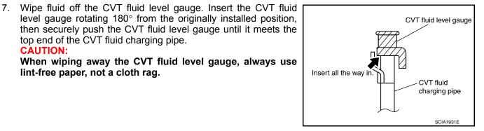
Place the selector lever in "P" or "N" and check that the fluid 8. level is within the specified range. **CAUTION:** When reinstalling CVT fluid level gauge, insert it into the
