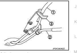
Install the selector cable (the M/T shift selector assembly side), as per the following procedure.
