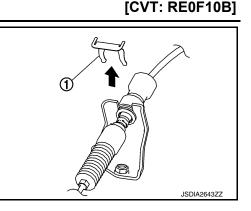
8. Remove the control cable (1) from the bracket (2).
