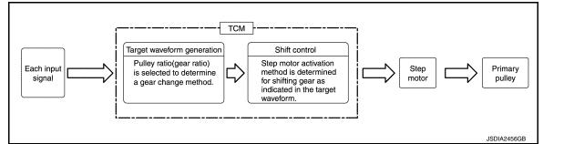
The gear ratio is set for each position separately.
