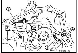
Temporarily install snap ring of mainshaft rear bearing into transaxle case.
