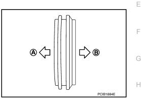
• Be sure not to hook center projection of 2 spread springs on same shifting insert.
