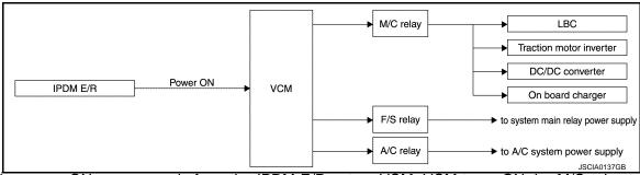
When the power ON power supply from the IPDM E/R enters VCM, VCM turns ON the M/C relay to supply power to each ECU in the EV system.
