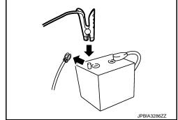
Before measuring the terminal voltage, confirm that the battery is fully charged. Refer to PG-96, "How to Handle 12V Battery".
