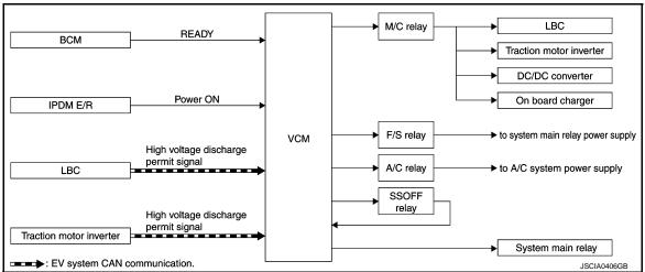
When the driver operates the POWER switch while depressing the brake pedal, VCM turns ON the M/C relay to supply power to each ECU in the EV system. Furthermore, VCM activates the F/S relay to start the power supply to the system main relay.
