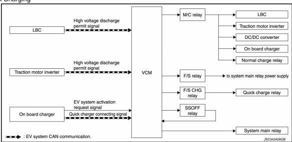
When VCM judges that the system is in quick charge mode, VCM turns ON the M/C relay to supply power to each ECU in the EV system. VCM also activates the F/S CHG relay to supply power to the quick charge relay inside DC/DC J/B. Furthermore, VCM activates the F/S relay to start the power supply to the system main relay.
