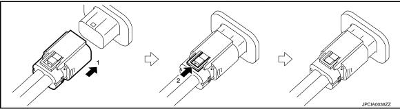
Follow the procedure below and connect the 3-step type high voltage harness connector.
