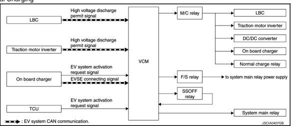
If VCM judges that the system is in normal charge mode, VCM turns ON the M/C relay to supply power to each ECU in the EV system and to the normal charge relay in the DC/DC junction box. Furthermore, VCM activates the F/S relay to start the power supply to the system main relay.
