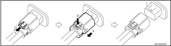
Follow steps shown below to remove a 3-step type high voltage connector.
