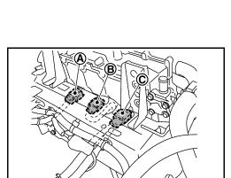
When disconnecting high voltage harness connector for electric compressor, disconnect it by inserting a suitable tool into inspection hole in traction motor inverter member.
