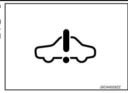
\*1: When the EV system warning lamp turns ON, it remains ON until the power switch is turned OFF. (Depending on diagnosis, the EV system warning lamp may turns OFF soon after the system returns to normal.)
