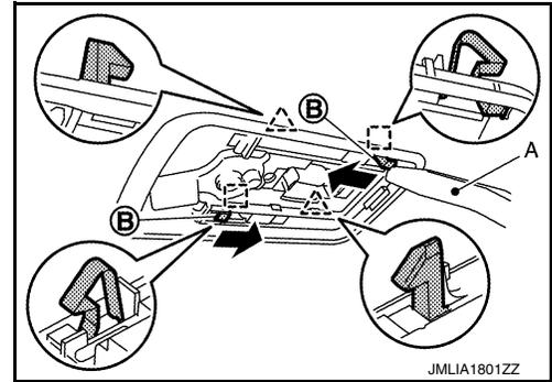
5. Disconnect the harness connector, and then remove room lamp assembly.
