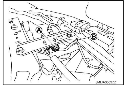
4. Disengage charge port light assembly fixing portion (A), and then push charge port light assembly, as shown (←).
