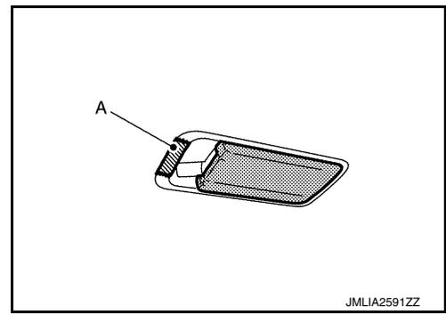
2. Disengage lens fixing pawls with a remover tool (A), and then remove lens.
