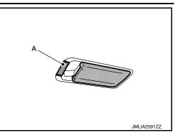
2. Disengage lens fixing pawls with a remover tool (A), and then remove lens.
