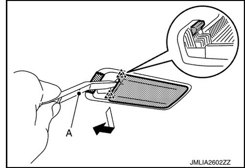
3. Using a remover tool (A), press the metal clip (B), and then disengage.
