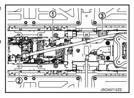
13. Remove the mounting nuts (A), and remove the bus bar (1) and high-voltage harness (2).
