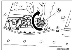
10. Install the Li-ion battery heater harness connector (A).
