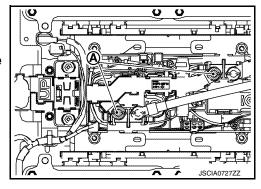
10. Remove the bus bar mounting nuts (A) and (B), and remove the bus bar (integrated with noise filter) (1).
