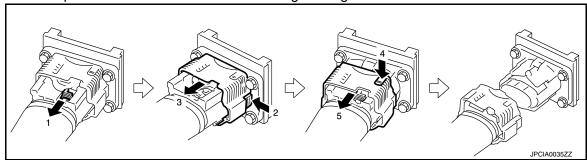
Disconnect the Li-ion battery heater harness connector (A).
