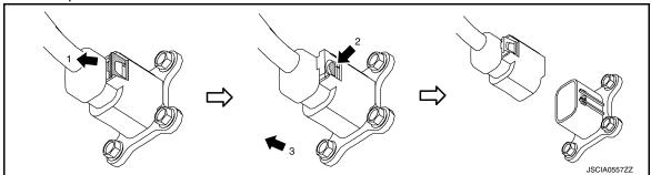
4. Disconnect the Li-ion battery vehicle communications connector (A) while rotating it in the counterclockwise direction.
