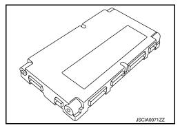
The LBC is the core of battery control. Li-ion battery controller detects the voltage and current of the assembled battery, the temperature of each module, and the voltage of each cell to judge state of charge. LBC also calculates possible input/output values, meter indication values, and chargeable values, and send this data to VCM (Vehicle control module). VCM controls the vehicle, according to the battery state.
