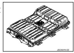
Four cells are integrated into a single module. The Li-ion battery consists of 48 modules placed in series.
