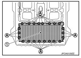
4. Tighten the mounting nuts (A), and then install the high-voltage harness (1), (2) onto the rear module stack.
