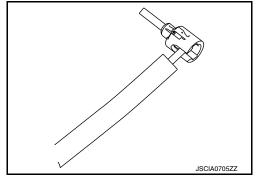
The sensor uses a thermistor with a resistance value that varies according to changes in temperature. The electrical resistance of the thermistor decreases as the temperature increases.
