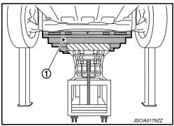
9. Remove the Li-ion battery mounting bolts (4 bolts) (A).
