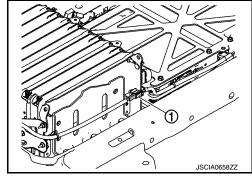
Remove the battery temperature sensor harness (front) ① from the front module stack RH.
