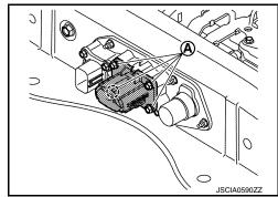
Disconnect the PTC heater harness connector (A).
