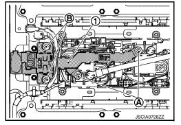
11. Remove the harness clips, then remove the battery member pipe ①.
