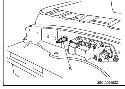
Install the gauge (A) of the air leak tester [SST: KV99111400 ( — )].
