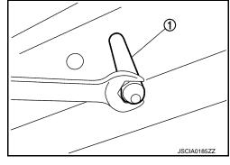
6. Install the Li-ion battery mounting bolts (A).
