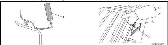
i. Insert a plastic remover tool (B) into the embossed locations to open a clearance.
