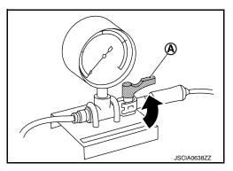
b. Operate the air pump slowly and apply the specified inspection pressure inside the battery pack. If the gauge pressure does not rise, or if the gauge reading fluctuates, check for the location of air leakage.
