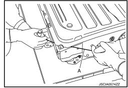
d. Use the windshield cutter (A) for cutting adhesive at the embossed locations.
