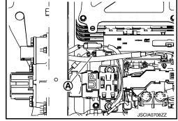
4. Open the bus bar cover and remove the high-voltage harness connector terminal mounting bolt (A).
