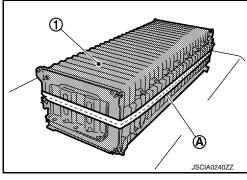
Inspect the module installation condition, and correct it if it is skewed or a large distortion is found.
