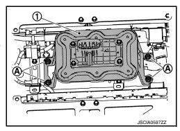
18. Invert the service plug switch bracket and remove the high-voltage harness mounting bolt ①, current sensor mounting bolt ②, and the connector ③, then remove the service plug switch bracket ④.
