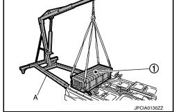
Move the battery pack and place the workbench below the rear module stack.
