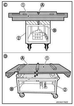
8. Set the pallet ① onto the Li-ion battery. CAUTION:
