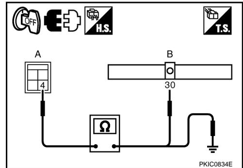
4. Check continuity between stop lamp switch harness connector (A) and ground.
