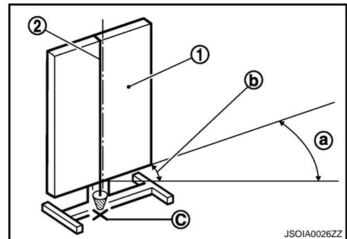
Check that the ICC target board (1) is located as shown in the figure.
