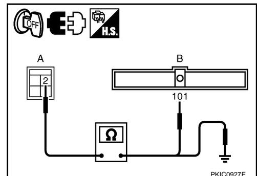
3. Check continuity between stop lamp switch harness connector (A) and ground.
