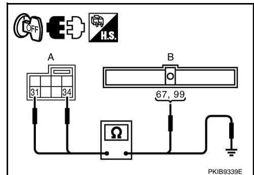
3. Check continuity between spiral cable harness connector (A) and ground.
