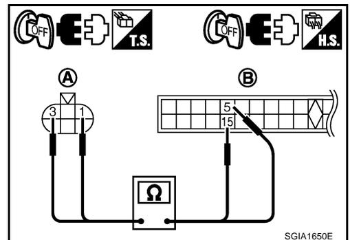
**4. CHECK REAR WHEEL STEERING ANGLE SENSOR OUTPUT SIGNAL**
