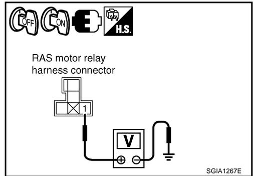
**Inspection 3: RAS Motor Output Malfunction**
