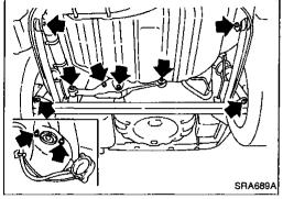
Retighten all nuts and bolts to the specified torque.
