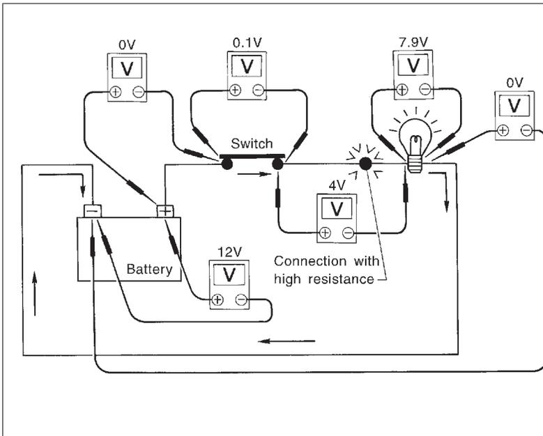
1. Connect the voltmeter as shown, starting at the battery and working your way around the circuit.
