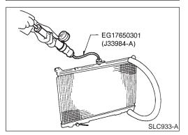
Apply pressure with Tool. Specified pressure value: 157 kPa (1.6 kg/cm<sup>2</sup>, 23 psi)
