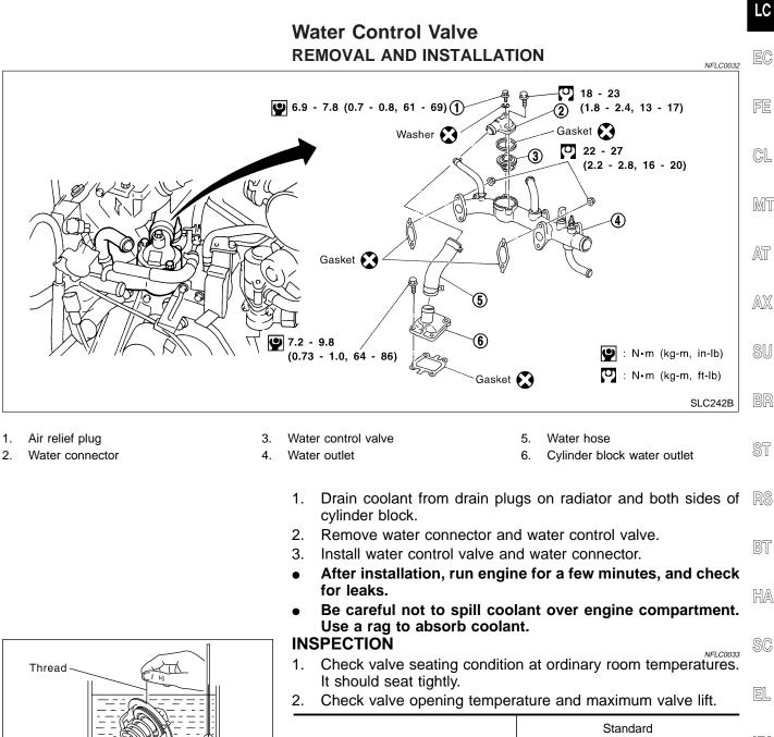
3. Then check if valve closes at 5°C (9°F) below valve opening temperature.
