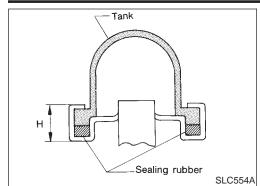
Make sure that the rim is completely crimped down.
