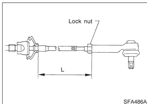
7. Adjust toe-in by varying the length of steering tie-rods.
