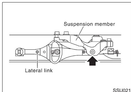
4. Using a transmission jack to lift the torsion beam, place lateral link and control rod horizontally against torsion beam. Tighten bolts and nuts to specified torque.
