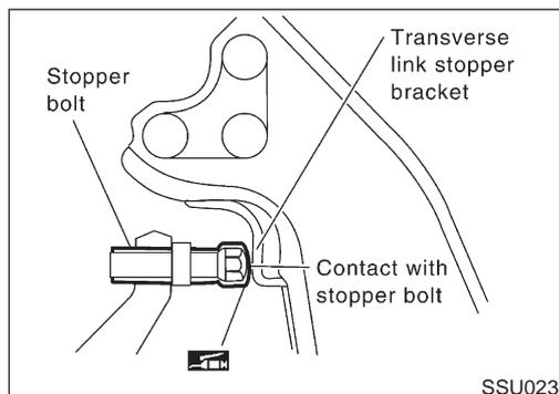
3. Check stopper bolt head to see whether it contacts stopper bracket at specified outside wheel angle. If not, adjust stopper bolt to contact stopper bracket at the correct angle. Adjust protrusion of stopper bolt before placing stopper bolt cap.
