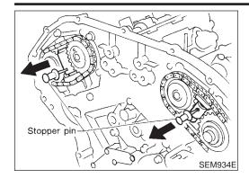
8. Remove RH and LH camshaft chain tensioner stopper pins.
