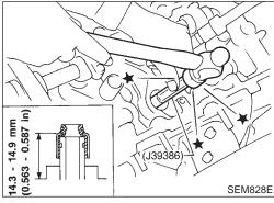
13. Apply engine oil to new valve oil seal and install it with Tool.
