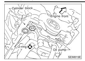
17. Remove O-rings from cylinder block and oil pump body.
