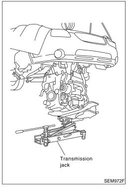
14. Remove engine with transaxle as shown.
