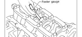
7. Measure connecting rod side clearance.
