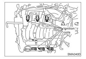
7. Remove RH and LH ignition coils.
