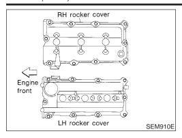
12. Remove RH and LH rocker covers from cylinder head.
