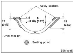
b. Apply sealant to front cover gasket and rear oil seal retainer gasket.
