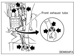
6. Remove front exhaust tube and its support. Refer to FE-10, "Removal and Installation".
