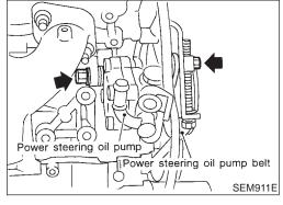
16. Remove power steering oil pump belt and power steering oil pump assembly.
