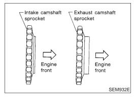
Be careful not to confuse intake and exhaust camshaft sprockets 2ND (their thicknesses are different).
