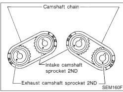
37. Remove exhaust camshaft sprockets 2ND, intake camshaft sprockets 2ND and camshaft chains on both sides.
