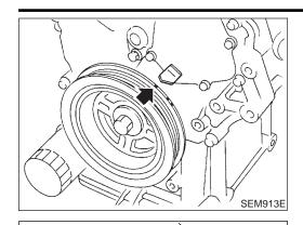
18. Set No. 1 piston at TDC on the compression stroke by rotating crankshaft.
