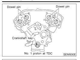
Position crankshaft so that No. 1 piston is set at TDC on compression stroke.
