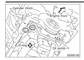
Install O-rings, cylinder block and oil pump body. e.
