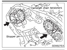
35. Attach a suitable stopper pin to RH and LH camshaft chain tensioners.
