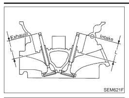
Use a depth gauge to measure the distance between the mounting surface of the cylinder head spring seat and the valve stem end. If the distance is shorter than specified, repeat step 5 above to adjust it. If it is longer, replace the valve seat with a new one.
