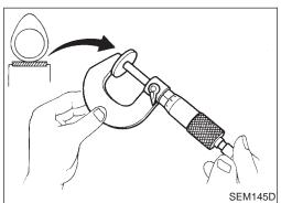
Shims are available in 64 sizes from 2.32 mm (0.0913 in) to 2.95 mm (0.1161 in), in steps of 0.01 mm (0.0004 in).
