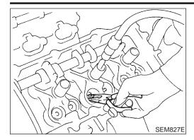
12. Remove valve oil seal.
