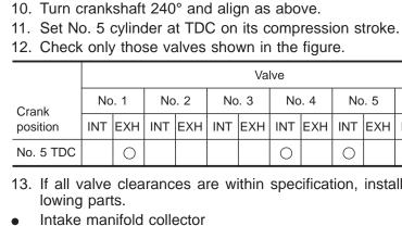
$\bigcirc$ 13. If all valve clearances are within specification, install the fol-
