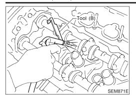
Blow air into the hole to separate adjusting shim from valve lifter.
