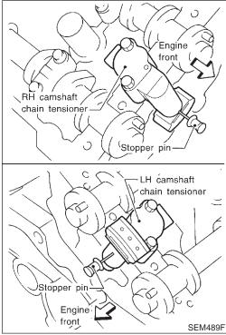
5. Remove RH and LH camshaft chain tensioners from cylinder head.
