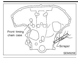
39. Use a scraper to remove all traces of liquid gasket from front timing chain case.
