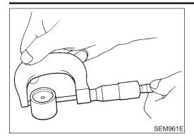
Check diameter of valve lifter and valve lifter guide bore. Valve lifter outer diameter:
