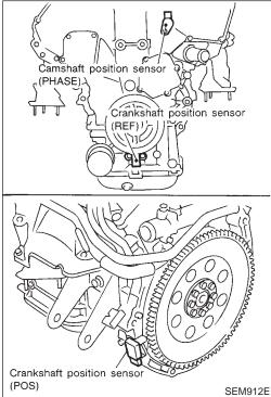
17. Remove camshaft position sensor (PHASE) and crankshaft position sensors (REF)/(POS).
