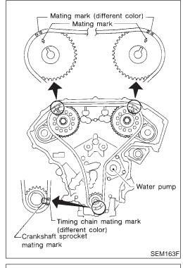
Align mating mark on crankshaft sprocket with matchmark on chain as shown.
