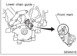
Install lower chain guide on dowel pin, with front mark on the guide facing upside.
