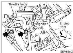
8. Remove intake manifold upper support bolts.
