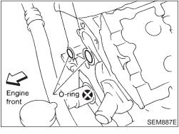
9. Install O-rings to cylinder block.
