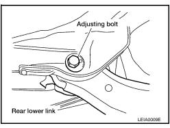
2. Tighten the adjusting bolt nuts to specification.
