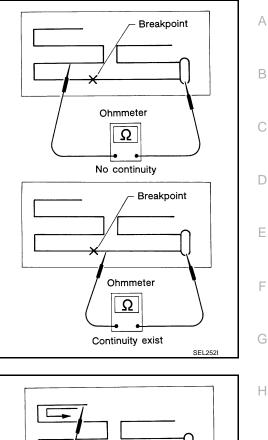
3. To locate a break, move probe along element. Tester indication will change abruptly when probe passes the broken point.
