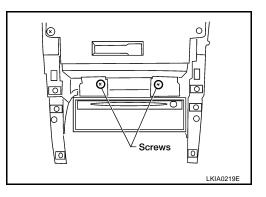
5. Pull carpet left of NAVI control unit aside and remove screws.
