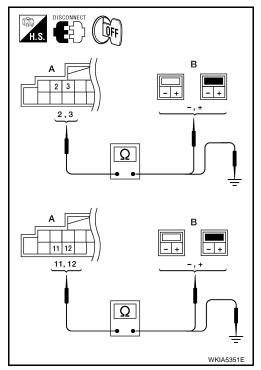
3. Check continuity between audio unit harness connector terminal and ground.
