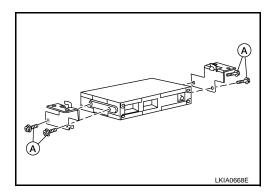
5. Remove satellite radio tuner.
