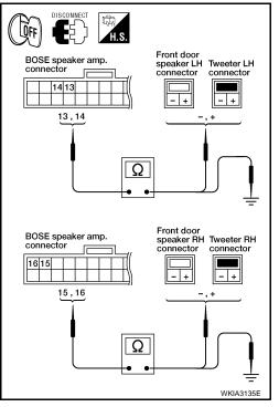
3. Check continuity between BOSE speaker amp. harness connector terminal and ground.
