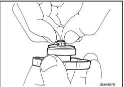
3. Check radiator cap relief pressure using Tool.
