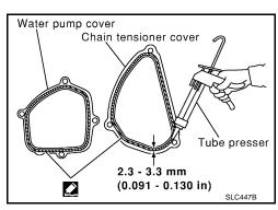
Apply a continuous bead of RTV Silicone Sealant or equivalent, b. to mating surface of chain tensioner cover and water pump cover. Refer to GI-46, "Recommended Chemical Products and Sealants".
