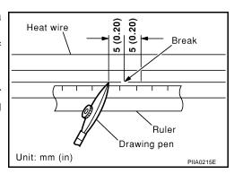
4. After repair has been completed, check repaired wire for continuity. This check should be conducted 10 minutes after silver composition is deposited.
