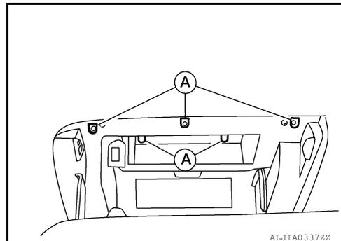
3. Remove the glove box assembly lower screws (A).
