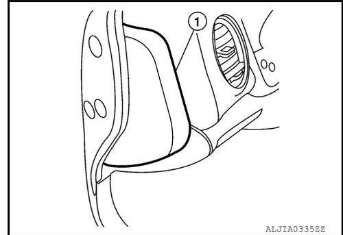
2. Remove the instrument lower panel (LH) (1).
