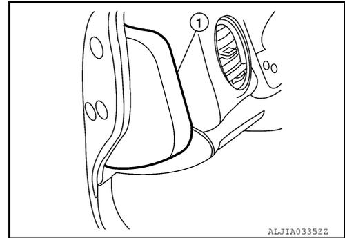
4. Remove the instrument lower panel (LH) (1). Refer to [IP-19, "Removal and Installation"](#).
