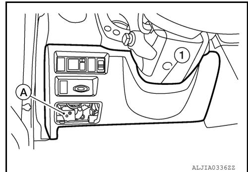
3. Remove cluster lid A screws, release the metal clips, and remove cluster lid A.
