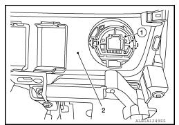
Release the pawl on each side and remove the NATS antenna amp (2) from the push-button ignition switch (1).
