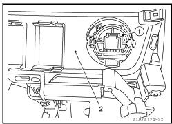
3. Release the pawl on each side using suitable tool and remove the push-button ignition switch (1) from the NATS antenna amp (2).
