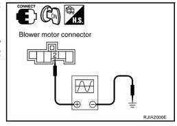
(L/Y) and ground using an oscilloscope. Usual No. 2 terminal drive signal duty ratios are shown in the table below.
