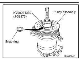
Using the holder to prevent clutch disc rotation, tighten the bolt to 14 N·m (1.4 kg·m, 10 ft-lb) torque. After tightening the bolt, make sure the pulley rotates smoothly.
