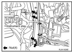
10. Remove mounting bolts from heater & cooling unit.
