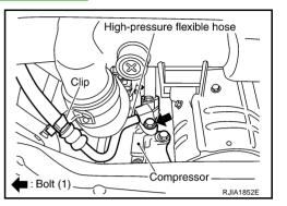
4. Remove the mounting nut for high-pressure flexible hose (Condenser side), and then remove the high-pressure flexible hose.
