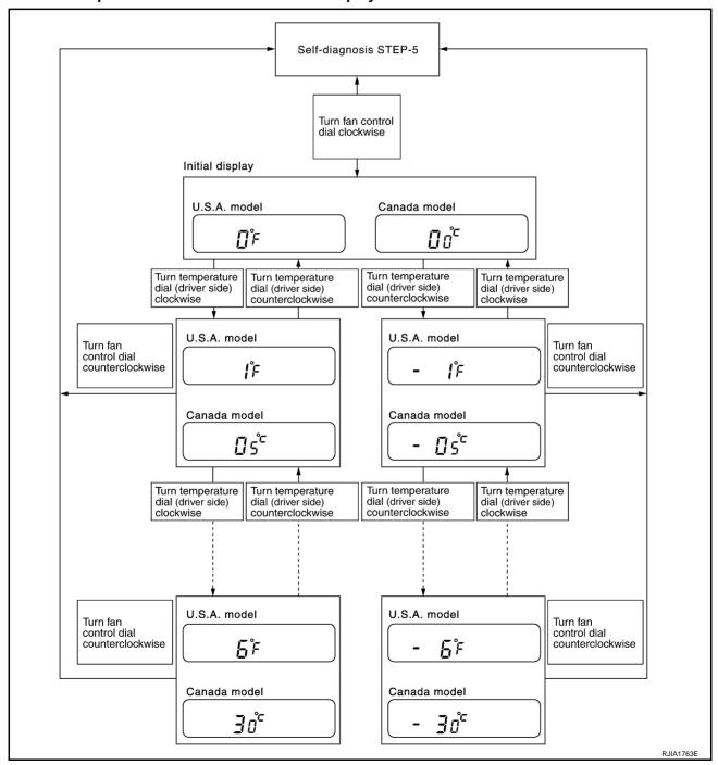
When battery cable is disconnected, trimmer operation is canceled. Temperature set becomes that of initial condition, i.e. 0°C (0°F).
