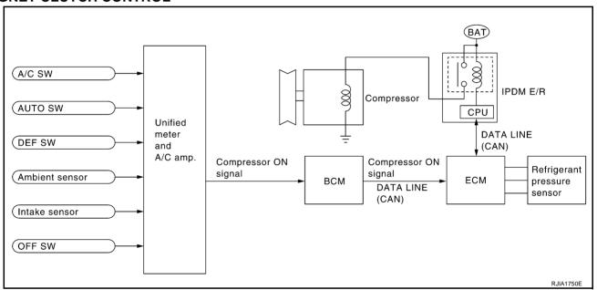
When A/C switch or DEF switch is pressed, unified meter and A/C amp. inputs compressor ON signal to BCM. BCM sends compressor ON signal to ECM, via CAN communication line.
