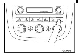
3. Confirm that discharge air comes out according to the air distribution table. Refer to <a href="ATC-31">ATC-31</a>, "Discharge Air Flow"</a>.
