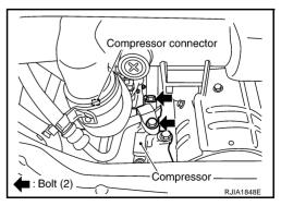
8. Remove engine oil hose bracket mounting bolt from compressor, using power tools.
