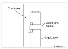
**Bolt mounting the liquid tank bracket (upper side)**
