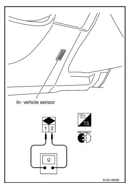
Unified meter and A/C amp. In-vehicle sensor connector
