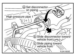
15. Remove the high-pressure pipe 1 mounting bolt, and then remove it.
