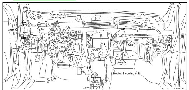
12. Remove the steering member, and then remove heater & cooling unit.
