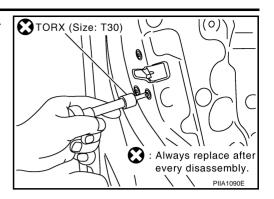
10. Remove the TORX bolt (T30), and remove the outside handle bracket.
