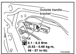
11. While pulling outside handle bracket, slide toward rear of vehicle to remove outside handle bracket.
