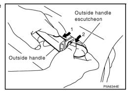
7. While pulling outside handle, slide toward rear of vehicle to remove outside handle.
