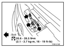
4. Disconnect the hood lock cable from the hood lock, and clip it from the radiator core support upper and hood ledge.
