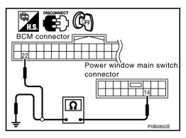
Check continuity between BCM connector M34 terminal 22 and front power window switch (passenger side) connector D35 terminal 16.
