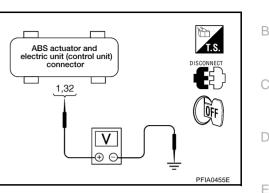
3. Check resistance between ABS actuator and electric unit (control unit) connector E24 and ground.
