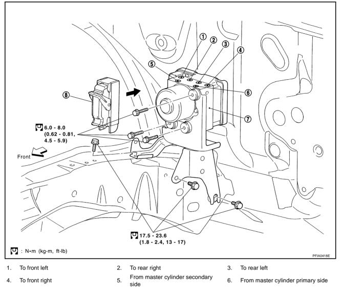
7. ABS actuator and electric unit (control unit) 8. Harness connector
