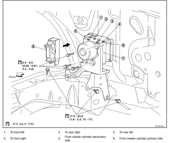
7. ABS actuator and electric unit (control unit) 8. Harness connector
