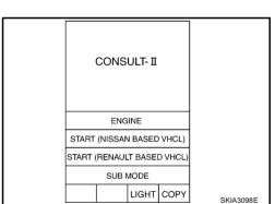
3. Touch "IPDM E/R" on "SELECT SYSTEM" screen. If "IPDM E/R" is not displayed, print "SELECT SYSTEM" screen, then refer to GI-39, "CONSULT-II Data Link Connector (DLC) Circuit".
