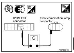
3. Check continuity between IPDM E/R harness connector E7 terminal 20 (R/Y) and front combination lamp RH harness connector E30 terminal 4 (R/Y).
