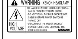
Do not touch the headlamp bulb glass surface with bare hands or allow oil or grease to get on it. Do not touch the headlamp bulb just after the headlamp is turned off, because it is very hot.
