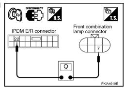
4. Check continuity between IPDM E/R harness connector and license plate lamp harness connector.
