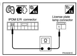
5. Check continuity between IPDM E/R harness connector and rear combination lamp harness connector.
