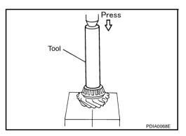
Drive Pinion Collapsible spacer
