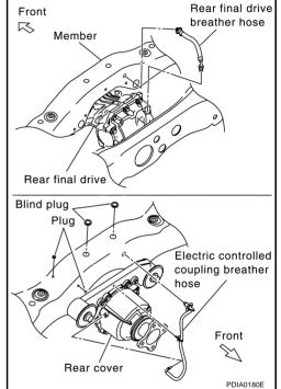
• Install metal connector of rear cover by inserting it with aiming blue painted marking to the rear of the vehicle.
