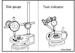
Rotate the drive gear back and forth in several times, check drive pinion gear to drive gear tooth contact.
