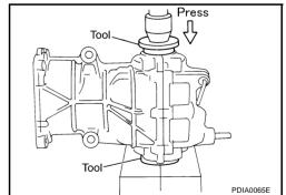
14. Fit a drift to the right and left side bearing adjusting shims individually. Compress differential case assembly and side bearing to install the rear cover.
