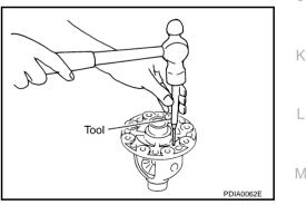
6. Using a drift, press a side bearing inner race into the differential case.
