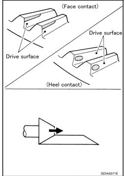
• In case of flank contact or toe contact, thin the drive pinion gear adjusting shims to move the drive pinion gear farther from the drive gear.
