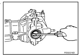
3. Fit a drift to the right and left side bearing adjusting shims individually. Compress differential case assembly and side bearing to remove gear carrier assembly and rear cover.
