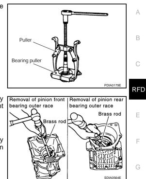
9. Using a brass rod, tap the pinion front bearing outer race evenly from the 2 cutouts on the gear carrier and remove pinion front bearing outer race.
