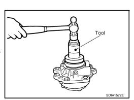
Using a drift and press in the companion flange.
