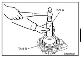
4. Using a drift, drive the adapter case oil seal until it becomes flush with the case end.
