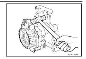
4. Using a flat-bladed screwdriver, remove the adapter case oil seal.
