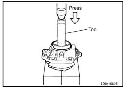
4. Using a drift, install the pinion front bearing outer race.
