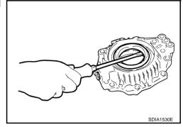
5. Using a brass rod, tap the gear ring bearing adjusting shim from the cutout on the adapter case to remove the gear ring bearing adjusting shim and gear ring bearing outer race.
