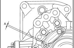
Using a drift, drive the transfer case oil seal until it becomes flush with the case end.
