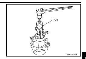
11. Using a puller, remove the pinion front bearing outer race.
