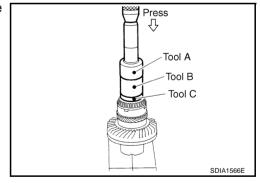
5. Apply gear oil to gear ring bearing inner race (adapter case side). Using a drift, install gear ring bearing inner race.
