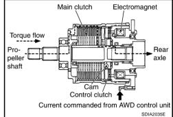
Transmission torque to rear wheels is determined according to command current.
