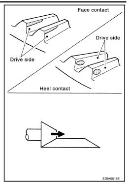
If the tooth contact is near the flank (flank contact), or near the toe (toe contact), thicken the pinion sleeve shims to move the drive pinion farther from the drive gear.
