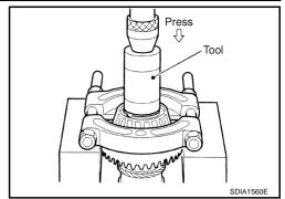
4. Using a drift and puller, remove the gear ring bearing inner race (transfer case side) on the gear ring.
