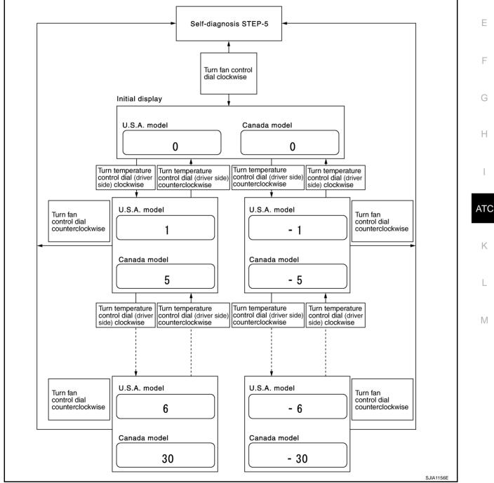
When battery cable is disconnected or battery voltage is below 10 V, trimmer operation is canceled. Temperature set becomes that of initial condition, i.e. 0°C (0°F).
