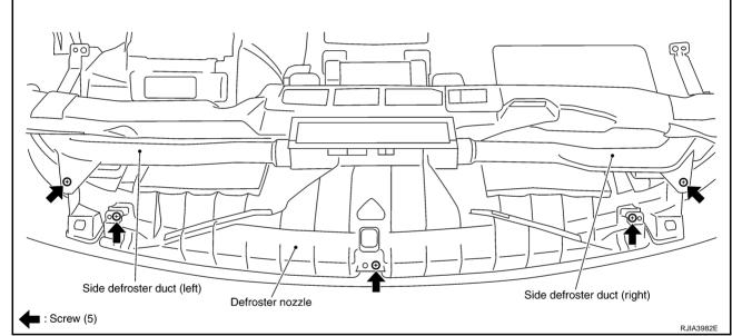
4. Remove mounting screws, and then remove ventilator duct, using power tools.
