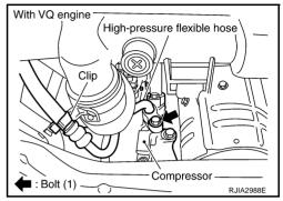
4. Remove mounting bolt from high-pressure flexible hose (Condenser side), and then remove high-pressure flexible hose.
