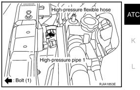
8. Remove mounting bolts, and then remove condenser. **CAUTION:**
