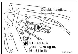
11. While pulling outside handle, slide toward rear of vehicle to remove outside handle.
