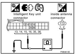
Check continuity between inside key antenna harness connector M102 (Console), M109 (dash board), B122 (luggage room) terminals 1, 2 and ground.
