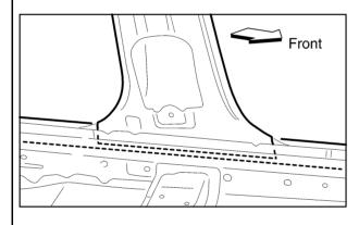
Install inner center pillar service part by putting between inner sill and outer sill reinforcement, then do M.I.G seam welding and M.I.G plug welding.
