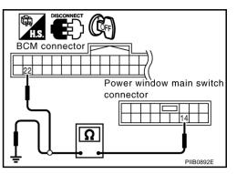
4. Check continuity between BCM connector M34 terminal 22 and front power window switch (passenger side) connector D35 terminal 16.
