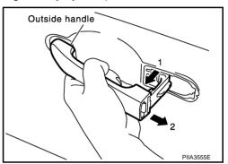
10. Remove the front gasket and rear gasket.
