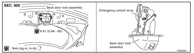
Remove the mounting bolts, remove back door lock assembly.
