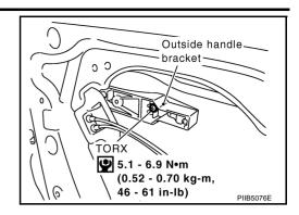
13. While pulling outside handle bracket, slide toward rear of vehicle to remove outside handle bracket.
