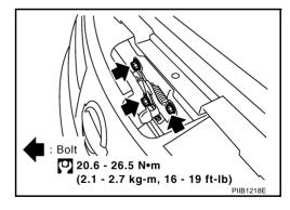
4. Disconnect the hood lock cable from the hood lock, and clip it from the radiator core support upper and hood ledge.
