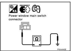
2. Check continuity between front power window switch (passenger side) connector D35 terminal 11 and ground.
