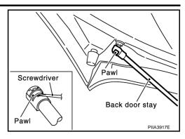
3. Remove back door stay assembly bracket adjusting nuts and remove back door stay assembly.
