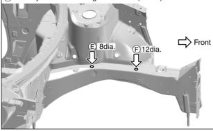
(e): Harness clamp installing hole center (8dia.)
