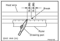
4. After repair has been completed, check repaired wire for continuity. This check should be conducted 10 minutes after silver composition is deposited.
