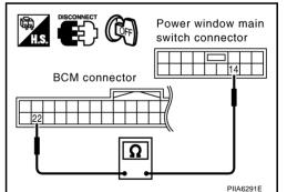
Check continuity between BCM connector M34 terminal 22 and front power window switch (passenger side) connector D35 terminal 16.
