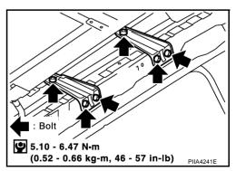
8. Remove sunroof unit assembly through the passenger compartment while being careful not to damage the seats and trim.
