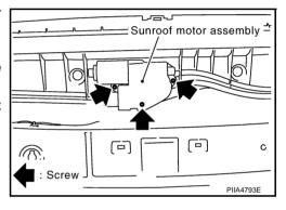
6. Remove nuts from the front end and side rail.
