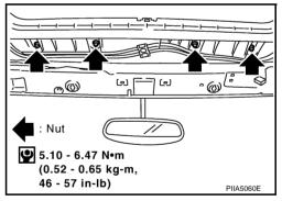
7. Remove sunroof bracket bolts, then remove sunroof unit assembly from roof panel.
