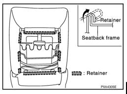
Squeeze and pull up headrest holder tabs to remove front seatback frame.
