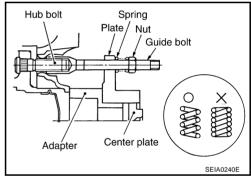
5. Place the dent of alignment gauge onto the projection of center plate and tightly contact them to measure.
