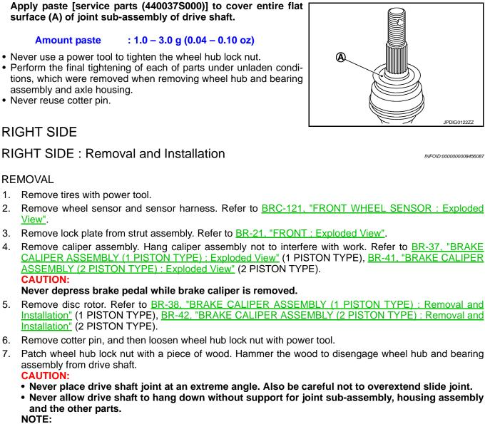
Use suitable puller, if wheel hub and bearing assembly and drive shaft cannot be separated even after performing the above procedure.
