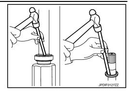
Install boot securely into grooves (indicated by "\*" marks) shown in the figure. CAUTION:
