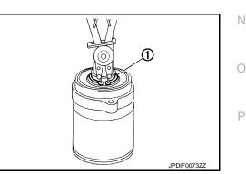
d. Install snap ring (1). **CAUTION:** Never reuse snap ring. [2WD]
