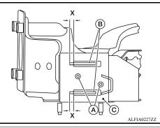
Overlap distance (X) between sub-bracket (B) and slide plate (C)
