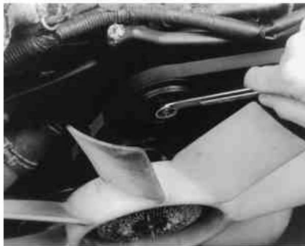
Fig. 8: Turn the adjusting bolt until the correct belt tension is achieved
