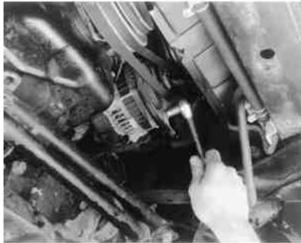
Fig. 5: Loosen the alternator pivot bolt with a box wrench or a ratchet and socket
