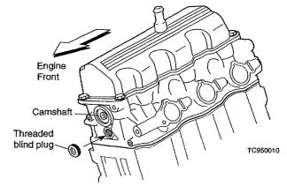
Prior to removing the timing belt, manually rotate the engine and align timing marks (this will ease re-assembly).
