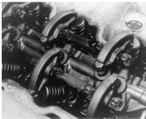
Fig. 12: After removing the rocker shaft assembly, keep all bolts in the proper order if possible
