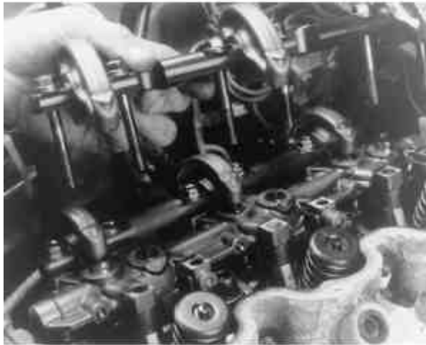
Fig. 13: Use a torque wrench when installing the rocker shaft assembly
