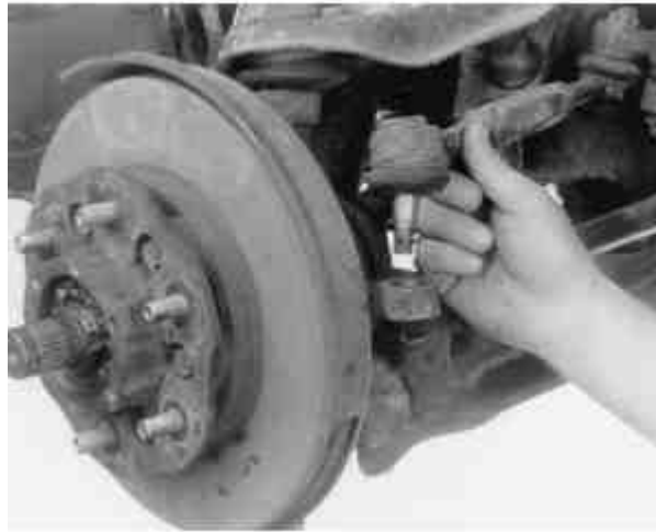
Fig. 13: Loosen the tie rod lock-nut after installing the tie rod into the spindle
