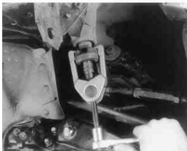
Fig. 6: Removing the pitman arm from the sector shaft — note arm is keyed for proper installation
