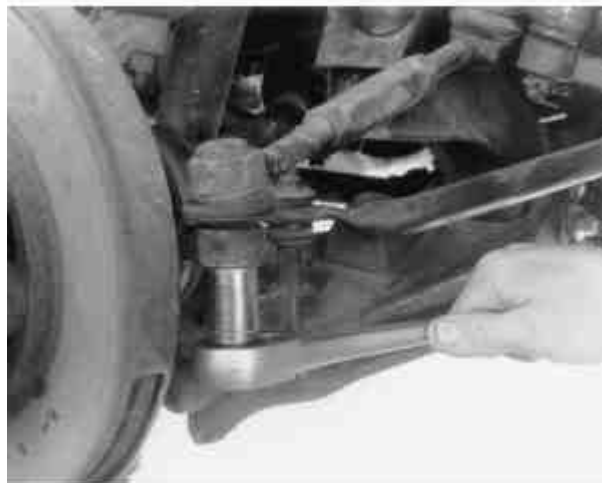
Fig. 11: Install the tie rod puller to remove the tie rod
