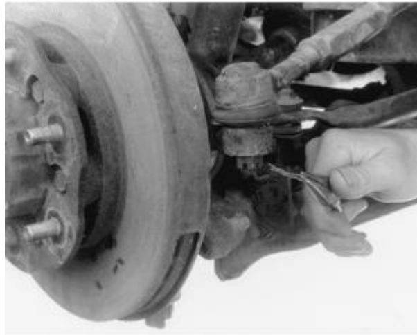
Fig. 10: Removing the tie rod assembly nut
