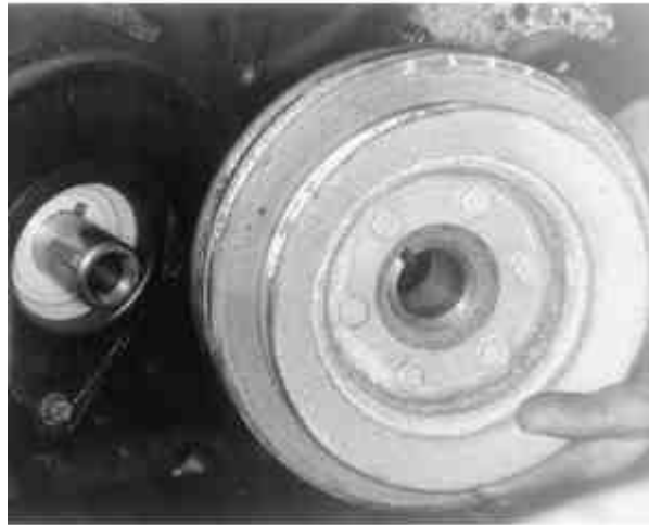
Fig. 5: Removing the lower timing belt cover
