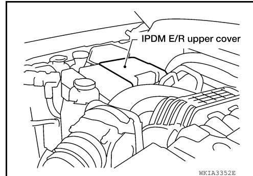
3. Release two clips and pull the IPDM E/R up from case.
