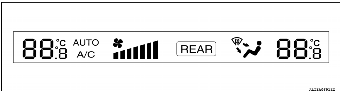
Controller (A/C switch assembly)
