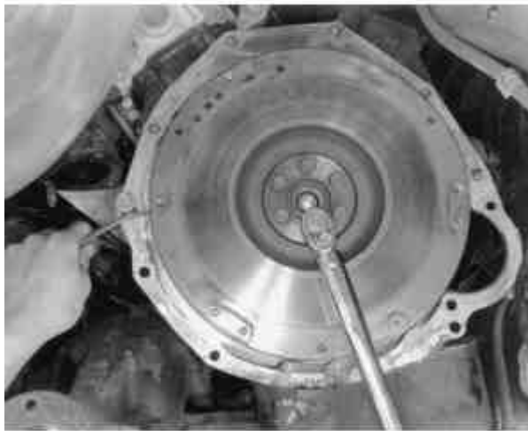
Fig. 12: Install the clutch assembly, make sure to tighten the retaining bolts in a crisscross pattern and lock the flywheel from turning
