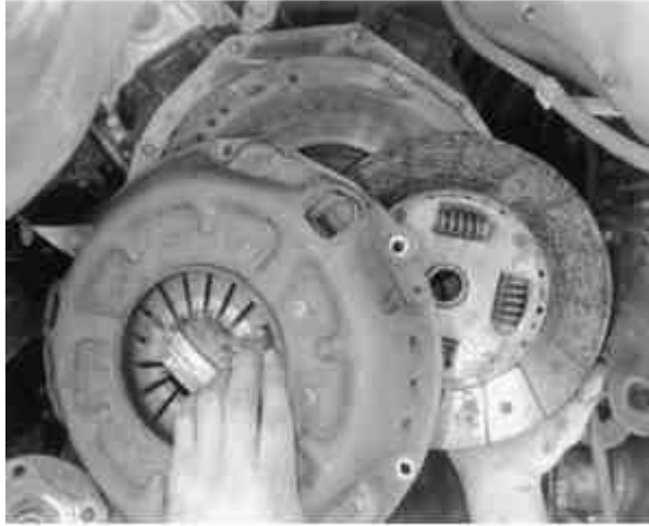
Fig. 9: When removing the flywheel assembly lock the flywheel from turning to aid in removal
