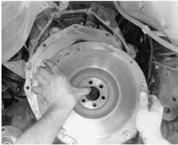
Fig. 11: Install the flywheel, make sure to tighten the retaining bolts in a crisscross pattern
