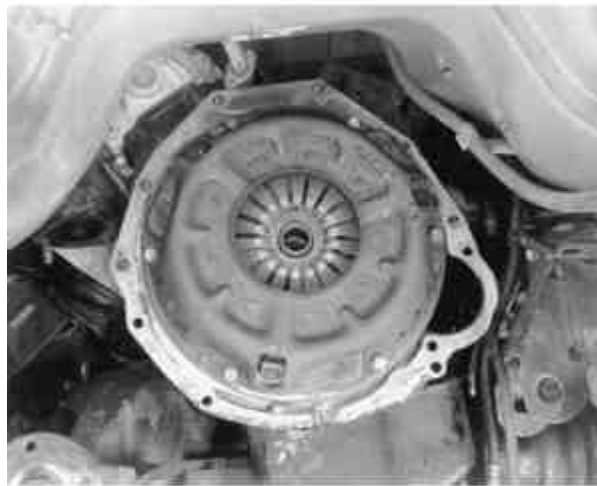
Fig. 6: Install a special aligning tool before removing the clutch assembly
