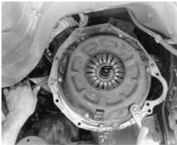
Fig. 8: View of the clutch pressure plate and disc assembly after the retaining bolts are removed
