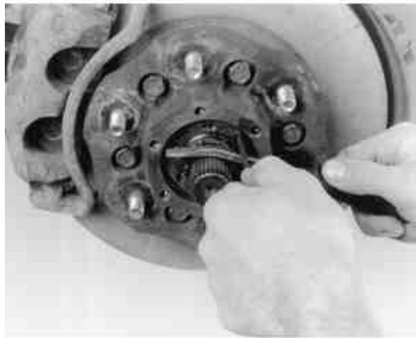
Fig. 17: After loosening the wheel bearing lock-nut remove the lock-nut from the hub assembly
