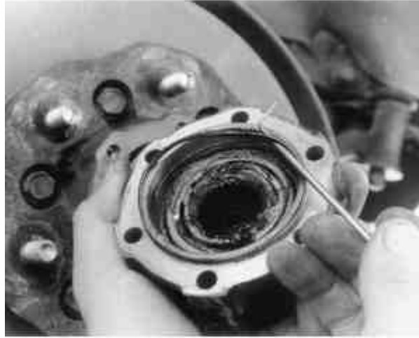
Fig. 10: Remove the snapring from the auto lock hub using snapping pliers
