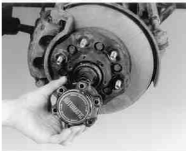
Fig. 9: Remove the auto lock hub housing then remove the O-ring, if necessary
