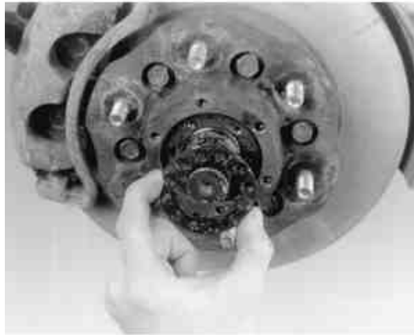
Fig. 16: Loosen the wheel bearing lock-nut — note position of tools used for this job
