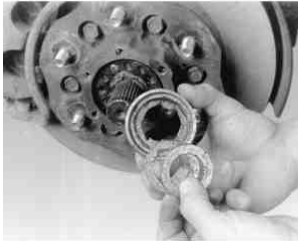
Fig. 14: After removing the auto lock hub assembly components remove the lock washer set screw
