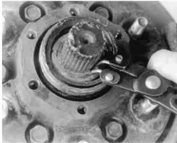
Fig. 12: Here the snapping is shown removed along with the spring, held up to show its relation in the assembly
