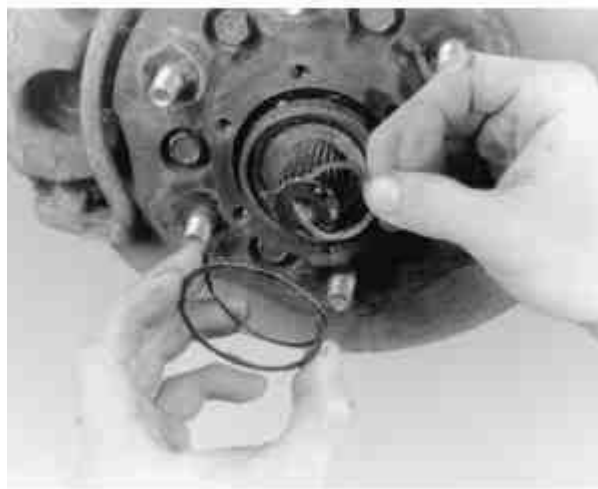
Fig. 13: Remove the washer and brake assembly, keep parts in order for correct installation
