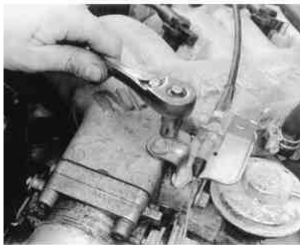
Fig. 6: Use a socket to remove the intake manifold collector mounting bolts
