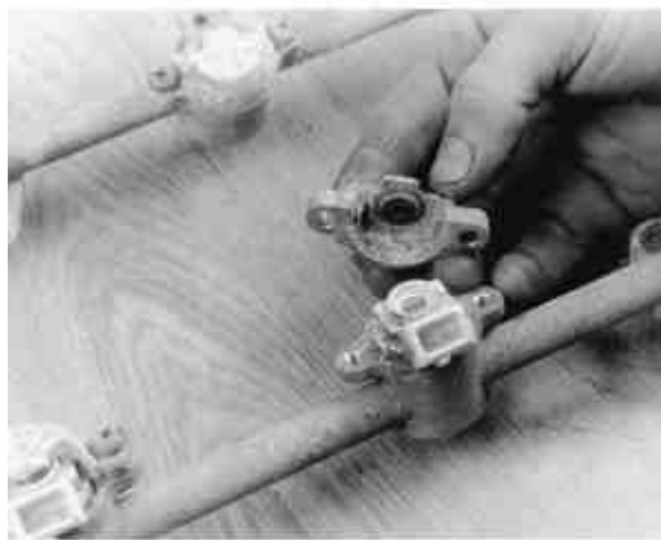
Fig. 18: Separate the injector from the fuel rail assembly
