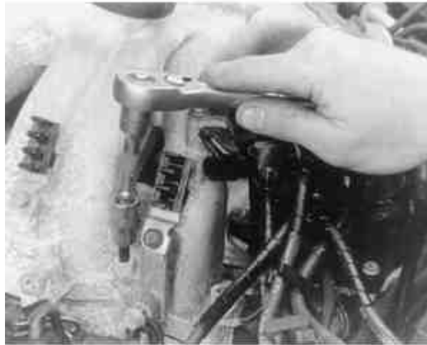
Fig. 9: Once the collector is removed, the fuel injector harness connectors are accessible
