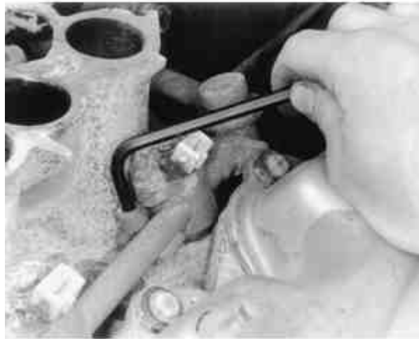
Fig. 15: Remove the fuel rail assembly from the engine with the injectors installed
