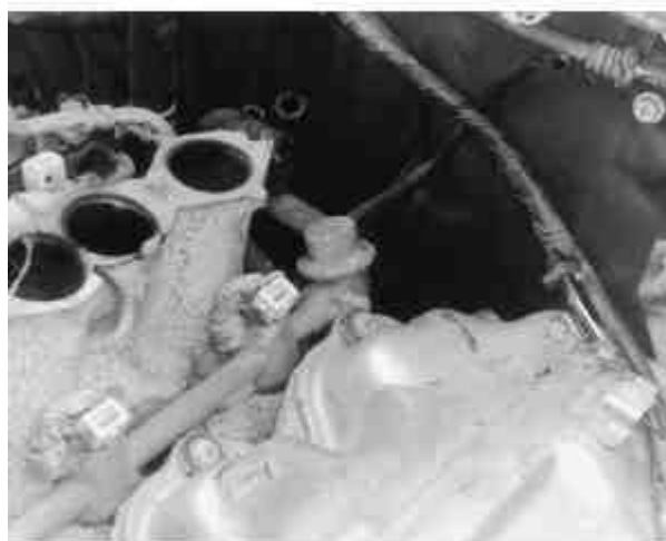
Fig. 14: Remove the fuel rail retaining bolts — use a hex-type socket or Allen key for this job
