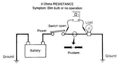
Unwanted resistance can be caused by many situations: -Undersized wiring (single strand)
