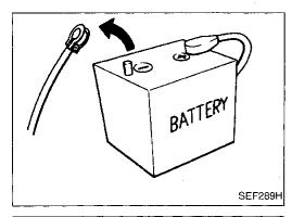
Before starting repairs which do not require battery power: Turn off ignition switch. Disconnect the negative battery terminal.
