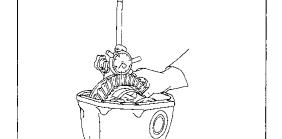
Measure ring gear to drive pinion backlash with a dial indicator.
