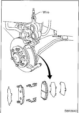
Open cylinder body upward. Then remove pad retainers, and inner and outer shims.
