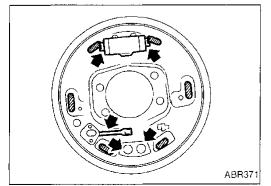
Apply brake grease to the contact areas (indicated by arrows and hatching) shown at left.
