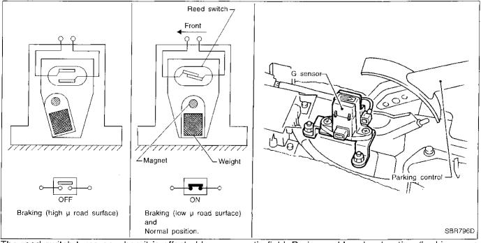
The reed switch turns on when it is affected by a magnetic field. During sudden deceleration (braking on a high  $\mu$  road), the weight moves and the magnet in the weight moves away from the reed switch. The magnetic field then diminishes and the reed switch turns off.
