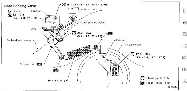
Tighten all flare nuts and mounting bolts.
