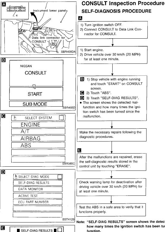
Note: "SELF-DIAG RESULTS" screen shows the detected malfunction and how many times the ignition switch has been turned since the malfunction.
