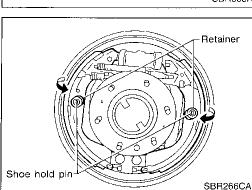
After removing shoe hold pin by rotating push retainer, remove leading shoe then remove trailing shoe. Remove spring by rotating shoes in direction arrow.
