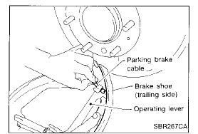
Be careful not to damage parking brake cable when separating it.
