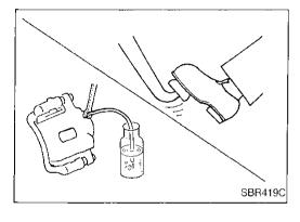
Connect a transparent vinyl tube to air bleeder valve.
