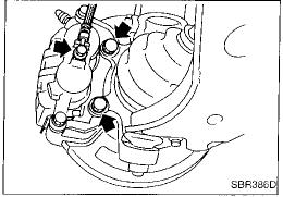
Remove torque member fixing bolts and connecting bolt.
