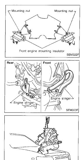
• Do not loosen front engine mounting insulator cover securing nuts.
