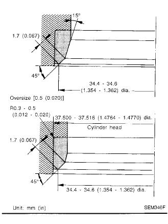
Inspection and Adjustment (Cont'd) CAMSHAFT AND CAMSHAFT BEARING
