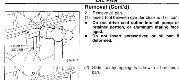
(2) Slide Tool by tapping its side with a hammer, and remove oil pan.
